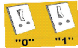
Figure 3.2 – A switch of an electronic circuit
